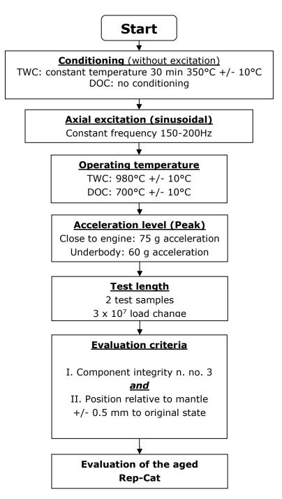
All temperatures are given as an average before / after substrate.
